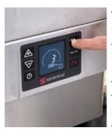
The FCS screen shows the force made by the motor at all times. It also enables an audible warning to be programmed for when the machine exceeds the established force. The user therefore obtains the desired cut quality in each product and at all times, achieving an optimum and uniform cut.
